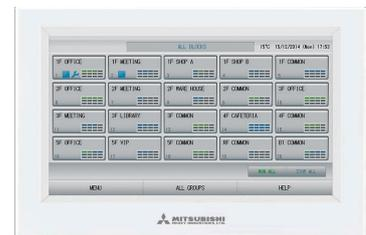
Easy operation realized with a large color LCD and touch panel. Up to 128 indoor units can be controlled, when SUPERLINK-II systems are connected.
